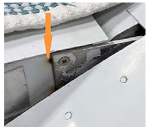
This Traveler's hinge nutplates have minor corrosion presenting on the rib, forward of the hinge, around the nutplate rivets.
